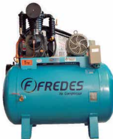
COMPRESOR 5 HP - 220V TRIF/BIF - 300 LTS - 175 PSI - 22 CFM
